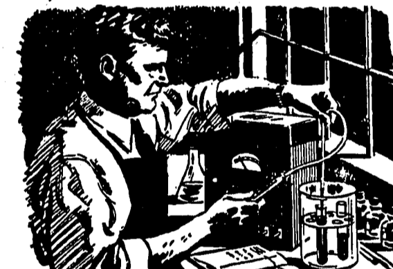
2. Geiger counters detected instantly the rate at which metal wore away from these atomically treated rings—under different circumstances, and with different oils!
