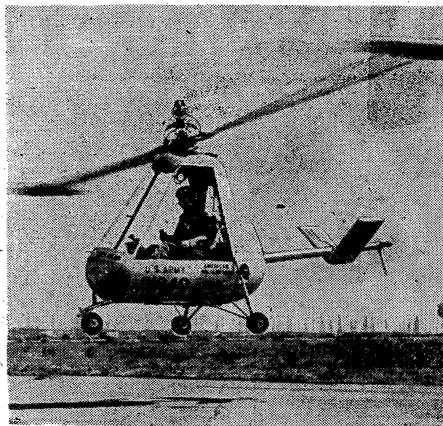
A one-man pulse-jet helicopter turned out for the U.S. Army zips into the air at Torrence, Calif., for a public flight demonstration. The small ship is designed for use by combat infantrymen and boasts a top speed of 80 miles an hour. It has been unofficially christened the "Jet Jeep" because of its jeep-like qualities in the air. The craft is the smallest 'copter ever procured by the US Army U.S. Army.
