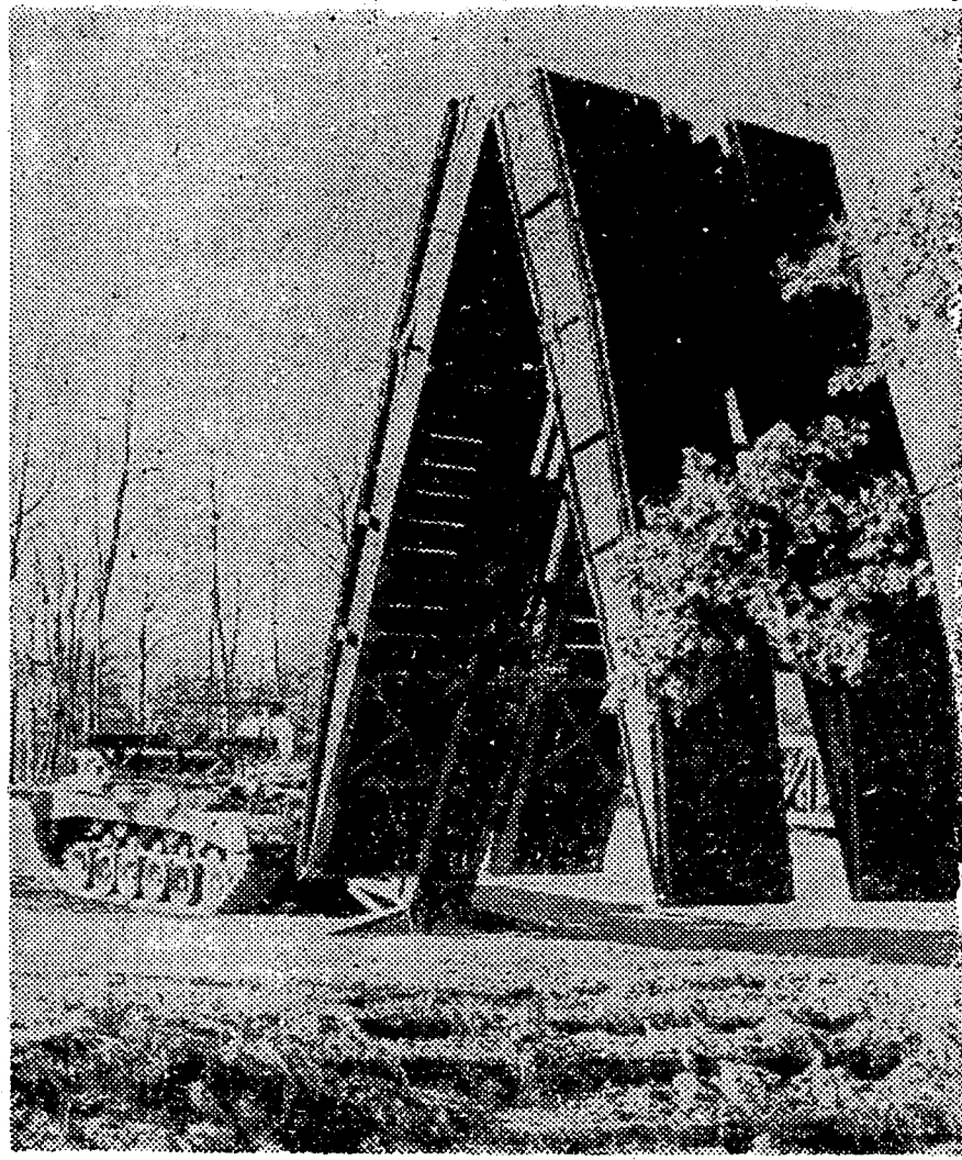
An experimental scissors-type bridge which is carried and launched by a turret-less tank, left, is demonstrated to a group of United States Army officers at Fort Belvoir, Va. Made of aluminum, the bridge is designed to carry loads up to 60 tons. Operated hydraulically it folds back over the tank for carrying.
